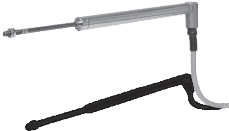
Fig. 4. 1-WA/200MM distance converter, before mounting on the test stand
