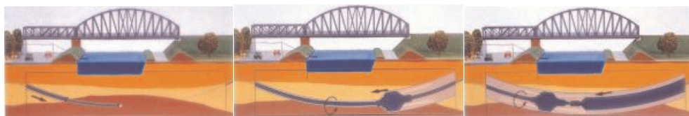
Fig. 1. Horizontal Directional Drilling. Source: Burkacki-Beta-Boring, Warsaw
