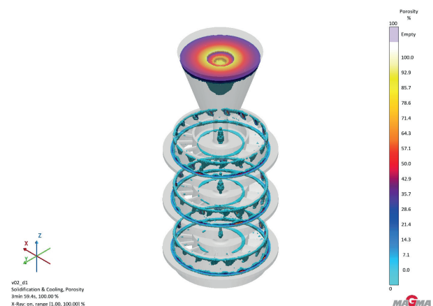
Fig. 13. Porosity distribution for the initial design (Design 1)
