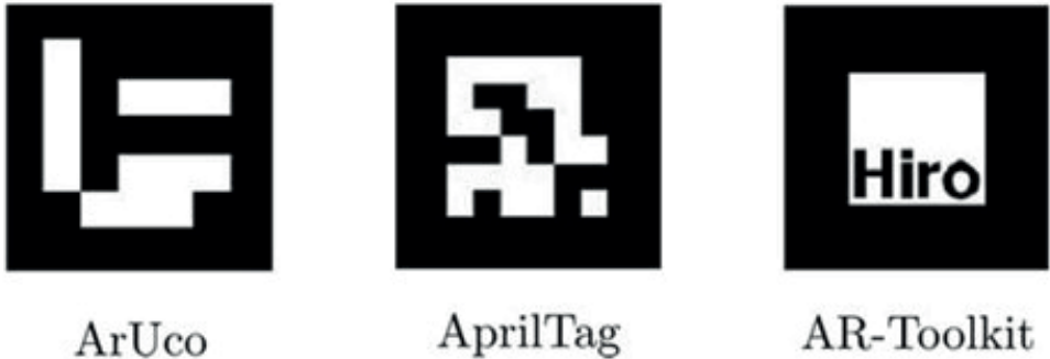
Fig. 8. Three examples of sign systems capable of generating fiducial patterns designed to be quickly located by machine vision systems (Botta, Quaglia, 2020)
