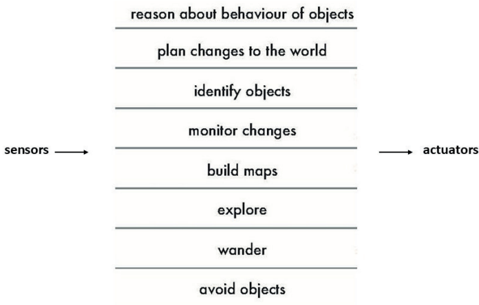
Fig. 16. A breakdown of the mobile robot system based on task achieving behaviours (after Brooks, 1985, Figure 2)
