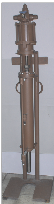
Fig. 8. Packer seal testing device
