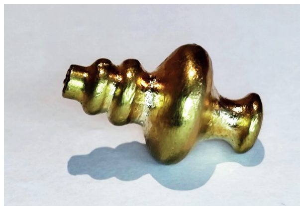
Fig. 9. Casting obtained using the investment casting method
