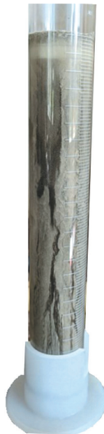
Fig. 7. Visualization of sedimentation stability breach of the grouting mortar
