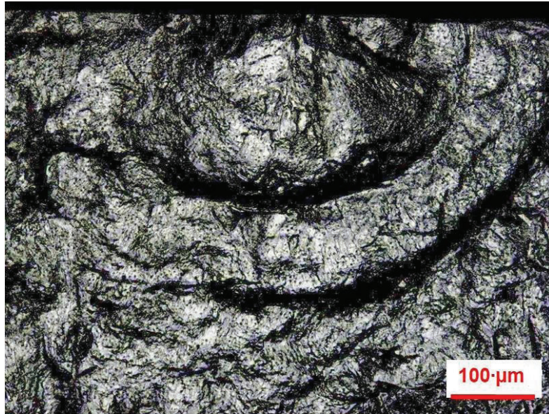
Figure 59. Fracture surface of a specimen tested in air at 400 °C after pre-annealing at 750 °C/150 h.
