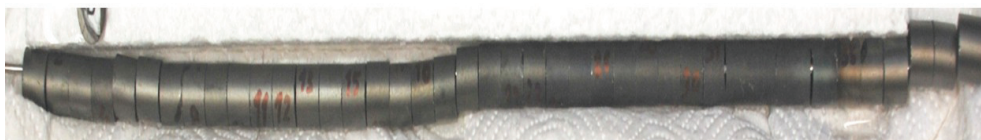
Figure 100. One of tube after operation sectioned in 10 mm width O-rings.
