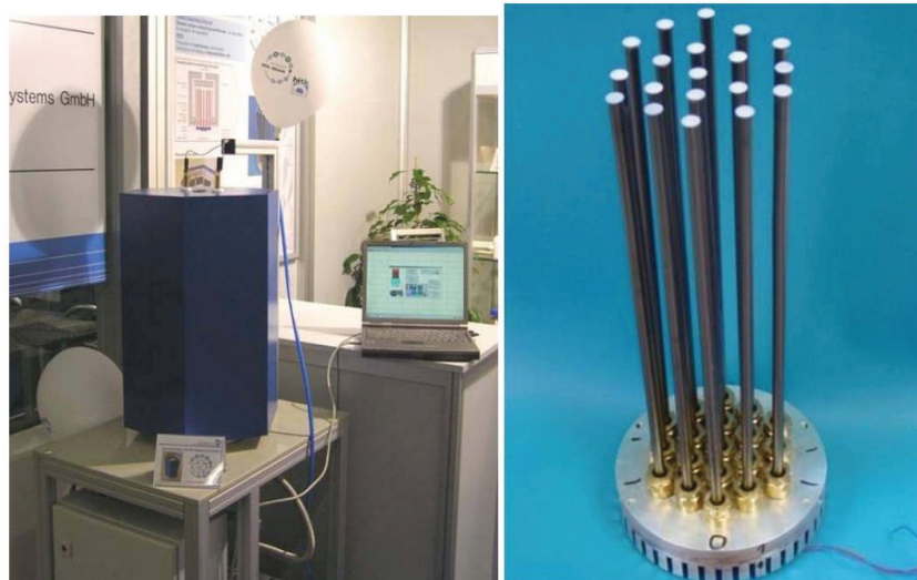
Figure 38. Demonstrator unit built up by the IKTS, Hermsdorf. a) Outer view of the system in operation. b) Array of tubular BSCF membranes mounted in a metal holder inside of demonstration unit [117].
