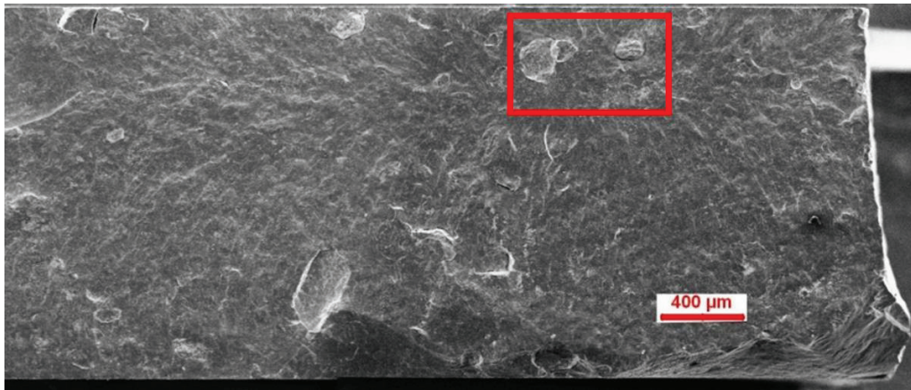
Figure 47. SEM image of fracture surface of a disc after ring-on-ring testing. The area marked by the red rectangle is shown in higher magnification in Figure 48.
