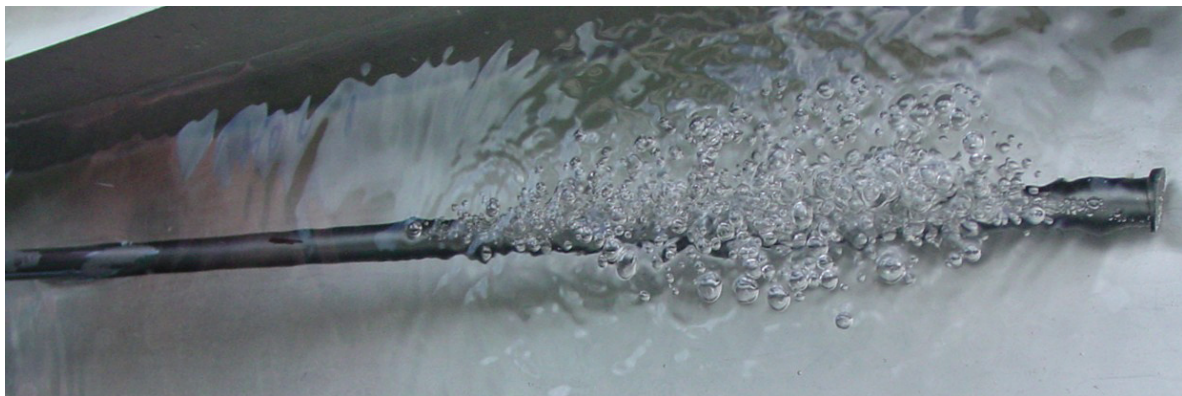
Figure 99. BSCF membrane tube fractured after operation during leakage test [courtesy of Voigt and Kriegel, IKTS].
