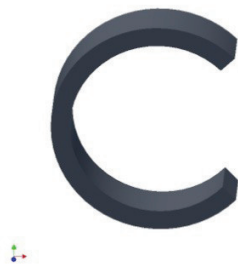
Figure 36. Geometry of C-ring specimen. \varnothing_0 = 15 mm, \varnothing_1 = 13 mm, t = 10 mm.
