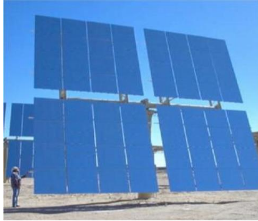
Figure 10. Example of single heliostat.
