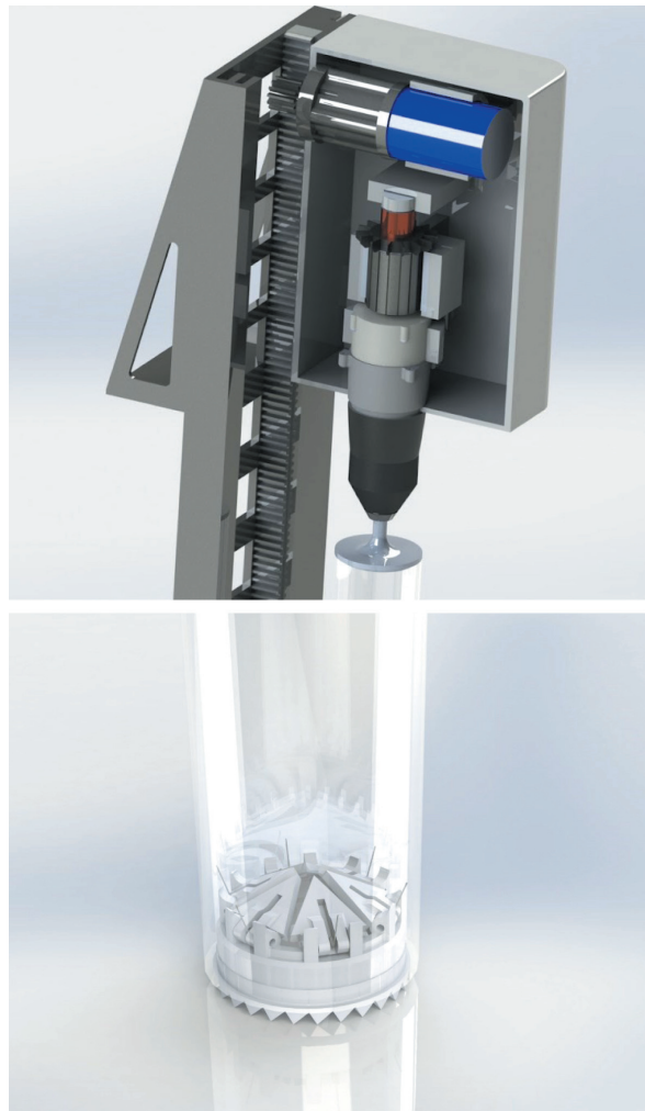
Fig. 4. Models of current versions of the mechanisms of the drill and core tube
