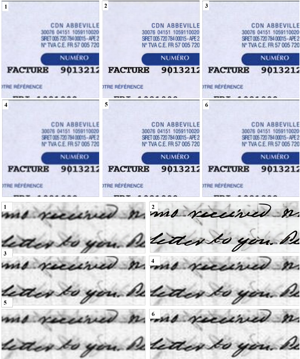
Figure 7. Visual comparison between our method and traditional methods: (1) LR image; (2) PSO.WESRGAN; (3) Bicubic; (4) Bilinlar; (5) Lanactoz; (6) Nearest Neighbor
