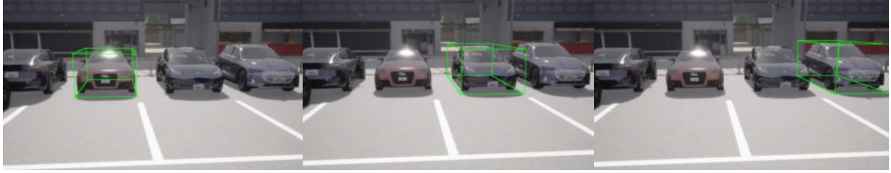
Figure 43: Example of automatically generated bounding box projection onto the camera image sensor data. Green lines depict the sized and position of each vehicle 3D label
