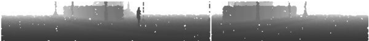
Figure 41: Range image generated out of the Carla simulation of LiDAR sensor, after the application of both post processing methods.
