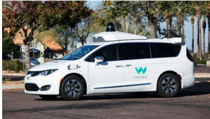
Figure 1: Waymo company vehicle equipped with five high quality cameras and five lidars.
