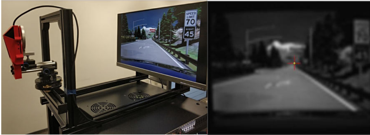
Figure 7: Left: HIL frame with Mobileye sensor and display attached. Right: Image stream out of the sensor from the same moment of time as on the left image.
