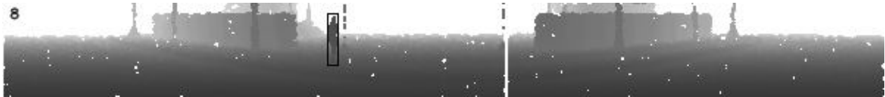
Figure 44: Example of automatically generated bounding box projection onto the LiDAR range image. Black box depicts the size and position of the pedestrian on the image.
