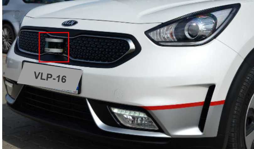
Figure 28: Smart Vehicle car equipped with Velodyne VLP-16 sensor.
