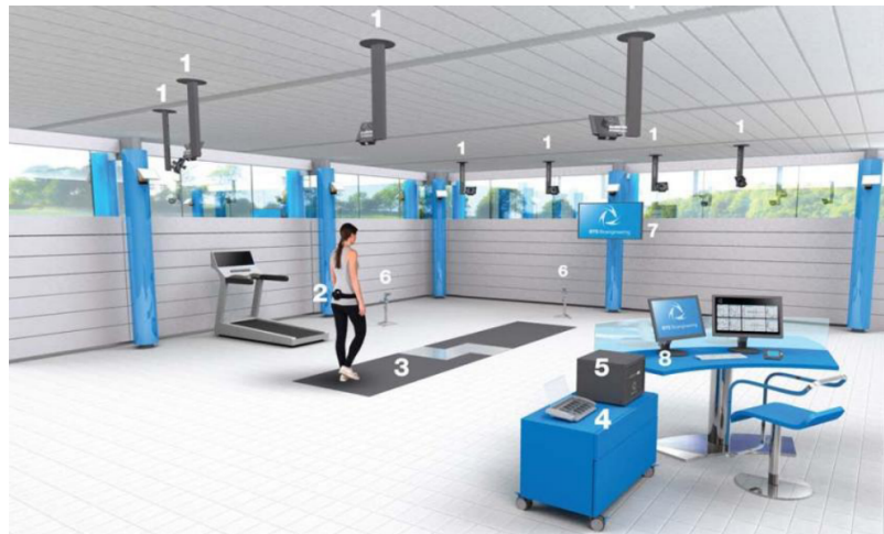
Fig. 3.8: Setup of a contemporary gait analysis laboratory (BTS Bioengineering, n.d.). (1) Infrared video cameras. (2) Inertial sensor. (3) GRF measurement gateway. (4) Wireless EMG. (5) Workstation. (6) Video recording system. (7) TV screen. (8) Control station.
