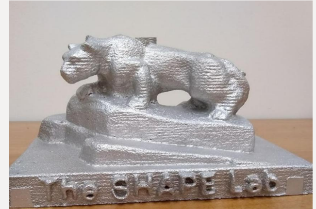
Figure 1. Casting made of aluminum alloy in a mold produced using binder jetting technology. [6]
