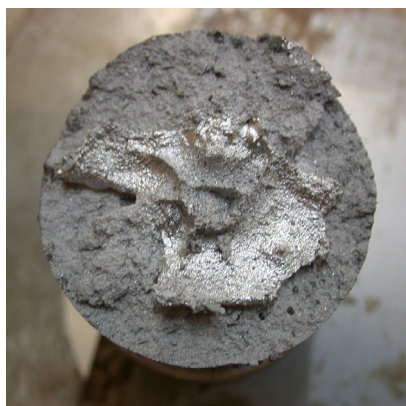
Fig. 8. Photo of the fracture of silumin AlSi21CuNiMg modified with AlCu19P1.4 (0.2%)
