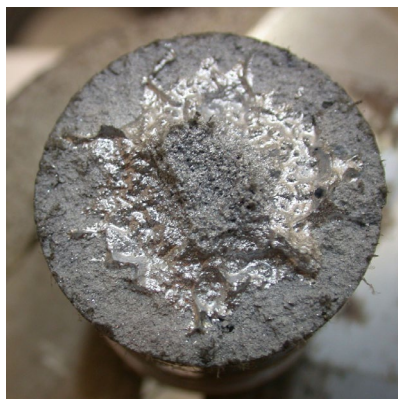
Fig. 7. Photo of the fracture of silumin AlSi21CuNiMg without modification
