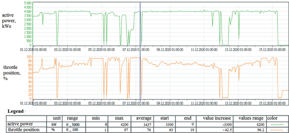
Fig. 6. Comparative graph of engine load and throttle opening rate after cleaning intake system and replacing flame arresters
