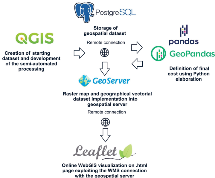
Fig. 3. Structure of WebGIS platform that integrates all blocks of chain with each other
