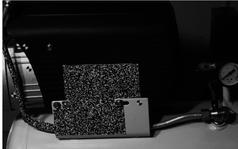
Figure 4.2: Representative video frame captured during the compressor experiment.
