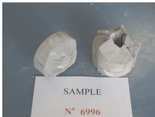
Fig. 8. Laboratory core plug N° 6966 (Fig. 7) photographed after destruction with a 3 g PCF propellant charge. Bottom part, broken by deflagration is shown at the left side. At right positioned fragment four fractures could be clearly noticed
