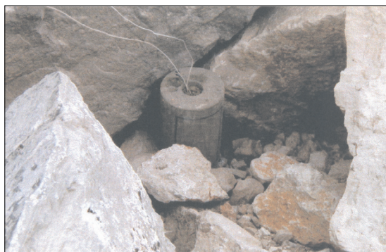
Fig. 7. Laboratory core plug N° 6966 photographed at polygon ready to be blasted by electrically activated a 3 g PCF propellant charge, positioned inside concentric hole
