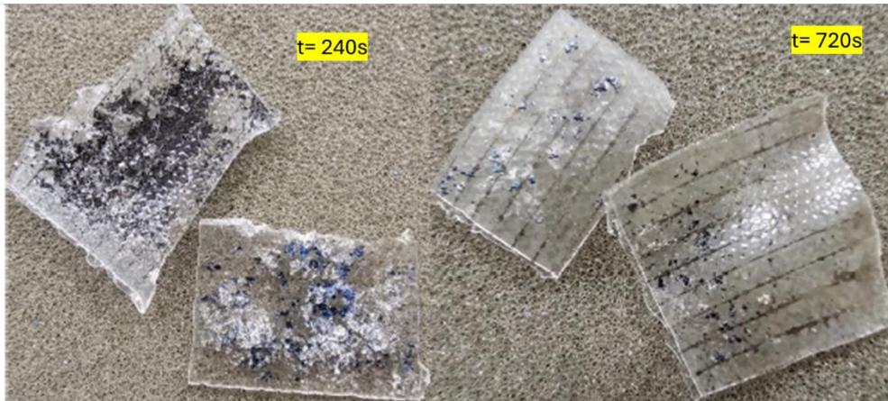
Figure 7: EVA pieces recovered from Glass-glass panel after a process duration of 240s (left) and 720s (right). The EVA pieces appear cleaner with less silicon sticking to the surface after longer process duration.
