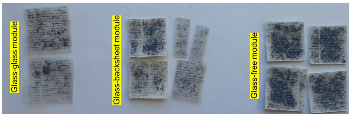
Figure 15 – Pieces of polymer recovered from the different panel types after the electrohydraulic treatment.
