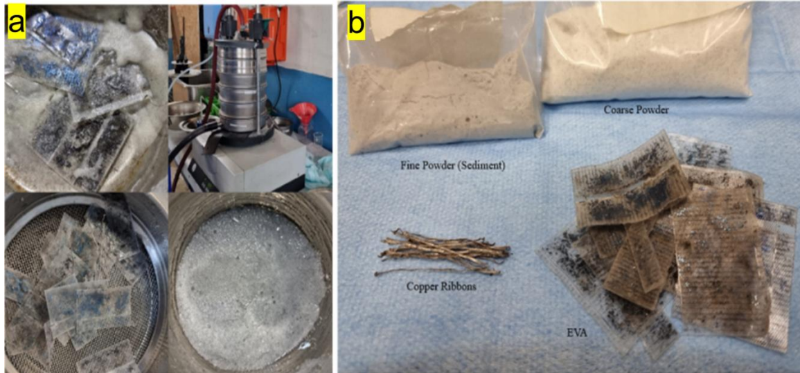
Figure 4: Recovered material after recycling a glass-glass panel using electrohydraulic processing a) Sieving and sorting the materials recovered b) the sorted materials recovered after drying.
