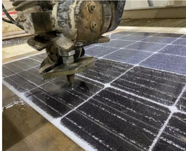
Figure 3: A glass-backsheet laminated PV panel being cut using the water jet cutting process.
