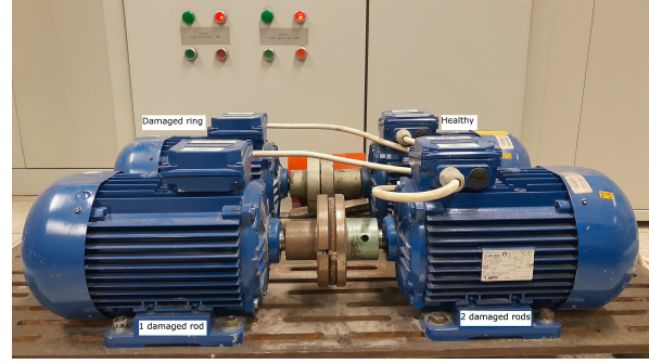
Fig. 1. Setup of four motors used for data collection. One of them was healthy, and the rest was damaged in different ways: broken rotor bar, two rotor bars broken, broken end ring. In this analysis, we focused on the broken rod diagnostics.
