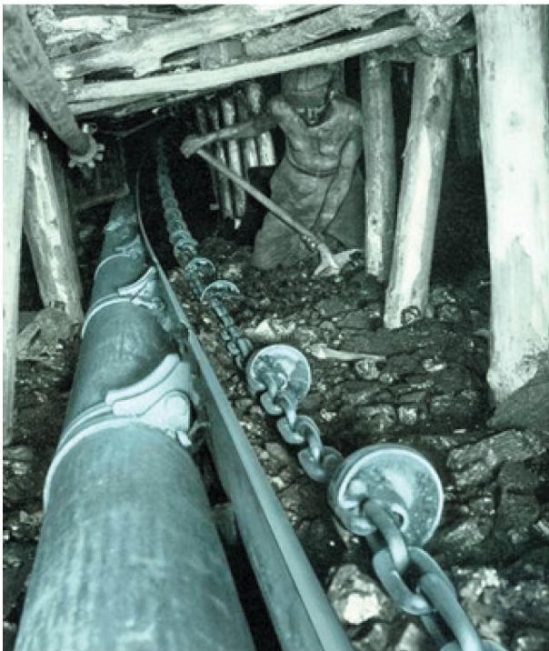
Fig. 2. Retarding disc conveyor
