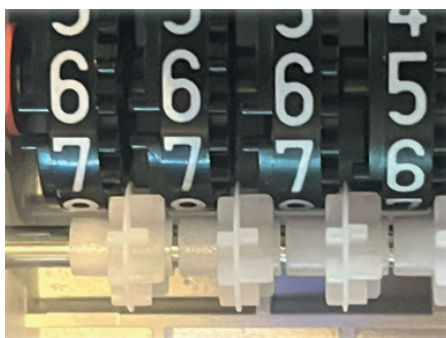
Fig. 15. Correct arrangement of the teeth of the decade flip-flops on the drums
