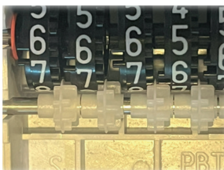
Fig. 16. Possibility of the slip-up of the wider tooth of the decade flip-flop into the space between the drums
