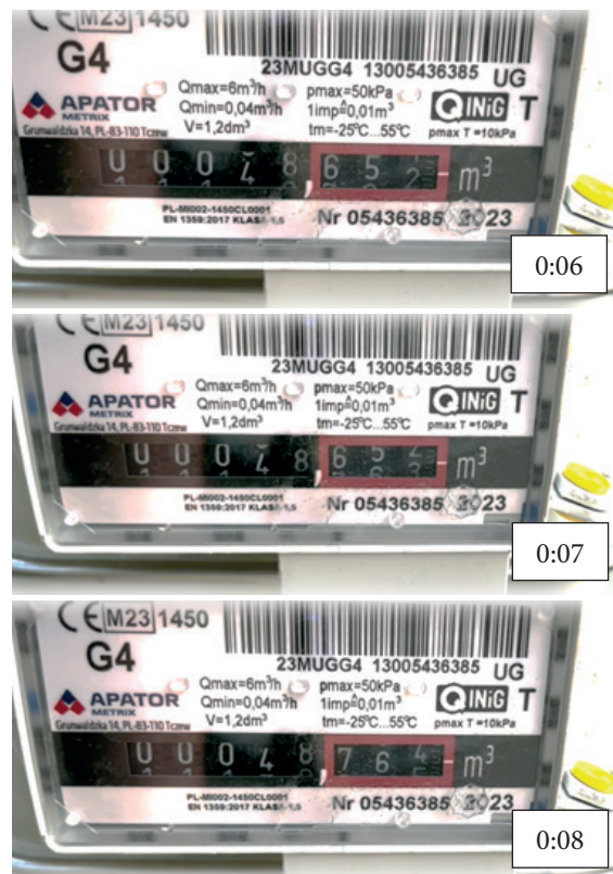
Fig. 21. Selected frames showing the counter jumping in a sealed gas meter
