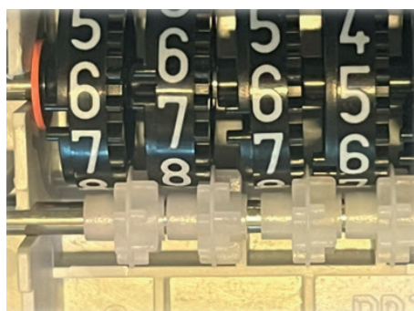
Fig. 17. Wider tooth of the decade flip-flop inserted between drums during rotation
