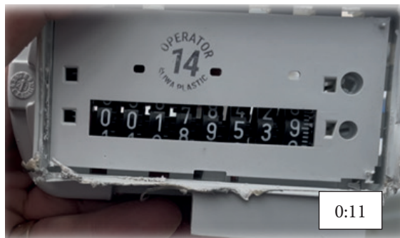
Fig. 5. Selected frames of a film showing the free rotation of the abacus drums
