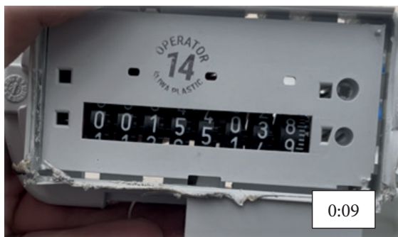
Fig. 5. Selected frames of a film showing the free rotation of the abacus drums
