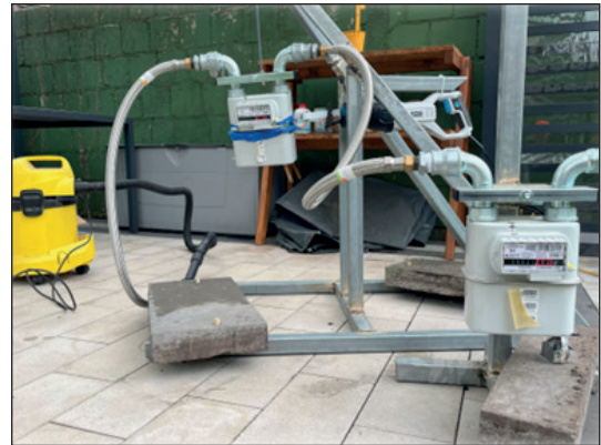
Fig. 3. Physical implementation of the measurement system based on an electric saw (1D vibration)
