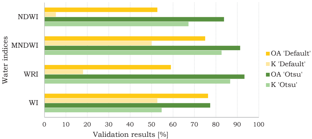
Fig. 4. Overall accuracies and kappa coefficients of NDWI, MNDWI, WRI, and WI based on reference data that was obtained from RPJMD 2019
