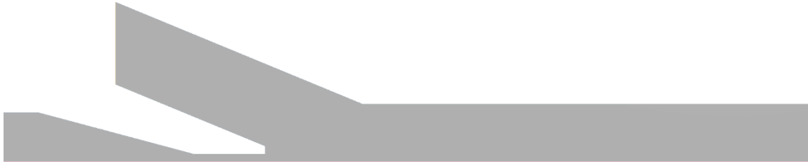
Figure 7.5. Axisymmetric, geometrical model of the spray-ejector condenser - nLPL variant, suction and mixing chambers.
