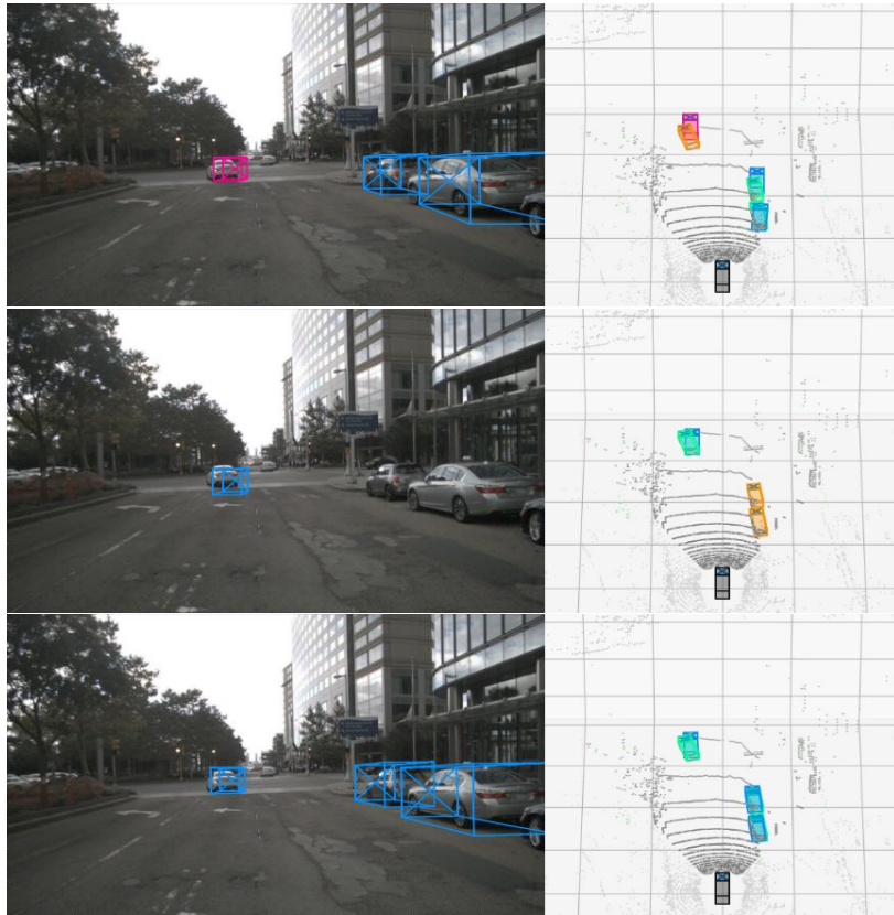
Figure 8.7: The example of a corner case scenario where the single sensor models for camera and Radar in the top and middle images, respectively, fail to produce accurate results. In contrast, the fusion model in the bottom image successfully combines the information from both sources and provides improved detection performance. The figure includes both the images and corresponding 3D views, accompanied by a visualization overlay that follows the established colour scheme.
