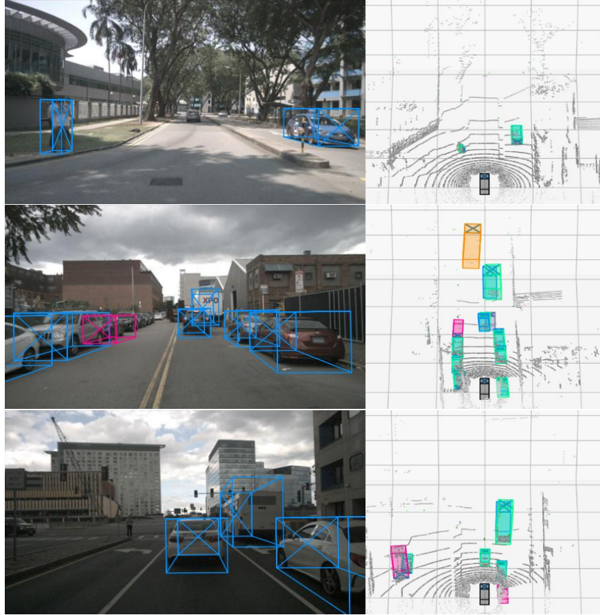
Figure 7.4: The results of LiDAR-only 3D OD model on NuScenes test set. The visualization specification matches the one used in Figure 7.3. The major difference could be observed in a LiDAR pointcloud data overlay. NuScenes sensor provides sparser detections within shorter ranges, which has a direct impact on the model performance at long-range detections.
