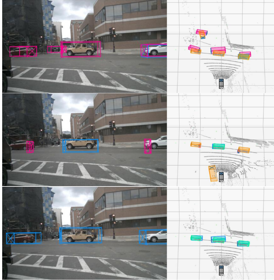
Figure 8.5: The comparison of the results for the same scene in the NuScenes test dataset, showcasing the outputs of the camera-only, radar-only, and CDSM fusion models from top to bottom. Both the images and corresponding 3D views are provided, along with a visualization overlay that follows the established colour scheme. In this colour scheme, labels are shown in green, positive detections in blue, false detections in magenta, and missed detections in yellow. The BEV also includes a LiDAR point cloud for reference. The presented image highlights the performance gain achieved through the fusion approach when compared to the single-sensor models.
