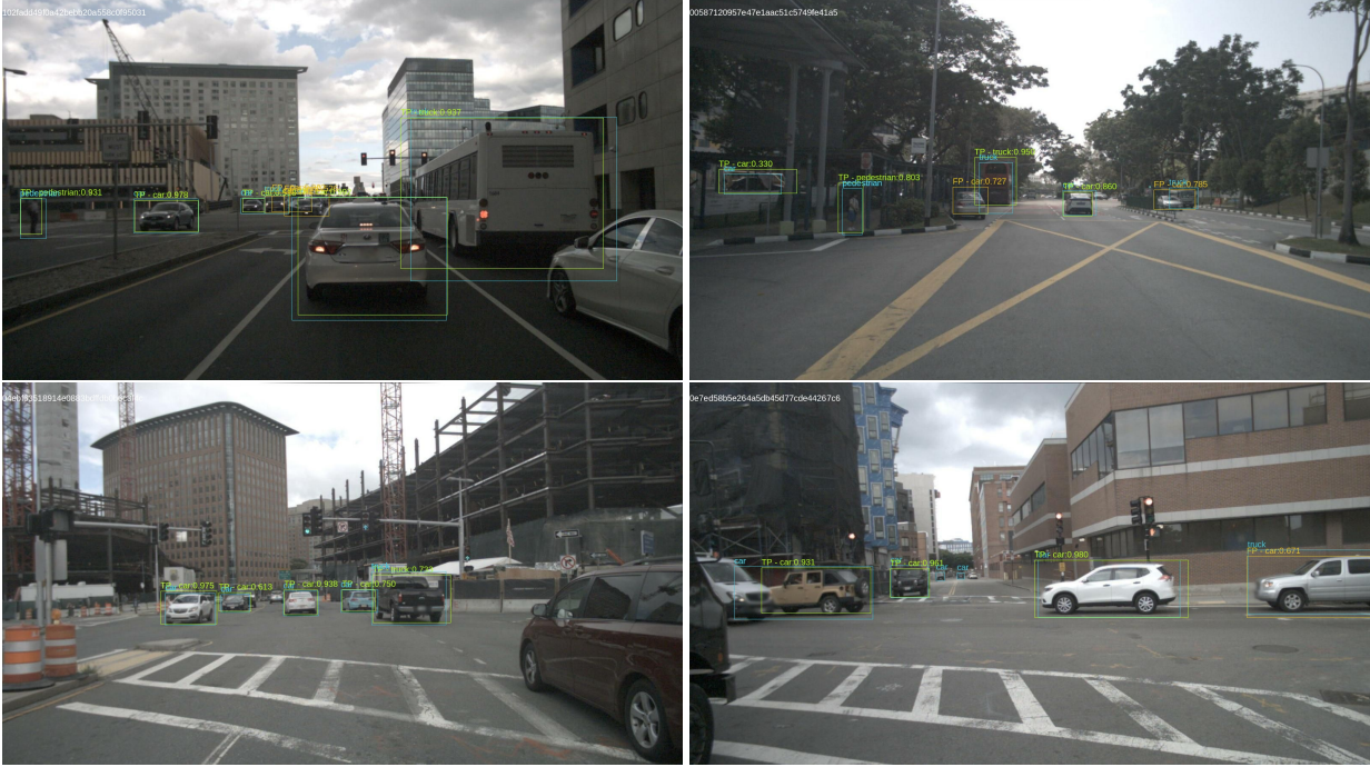
Figure 7.2: The results of camera-only 2D OD model on NuScenes dataset test image samples. Labels and predictions overlay presentation are consistent with the one used in Figure 7.1. Additionally, orange "FP" bounding boxes represent False Positive detections, not associated with any labelled objects.
