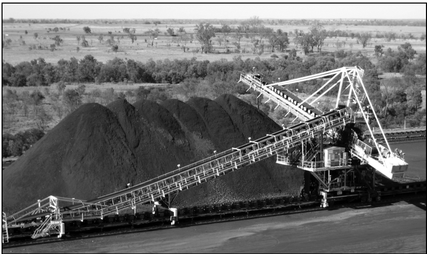
Fig. 3. Krupp coal stacker featuring tripper conveyor and non-slewing, luffing boom at RTCA Kestrel Mine [4]
