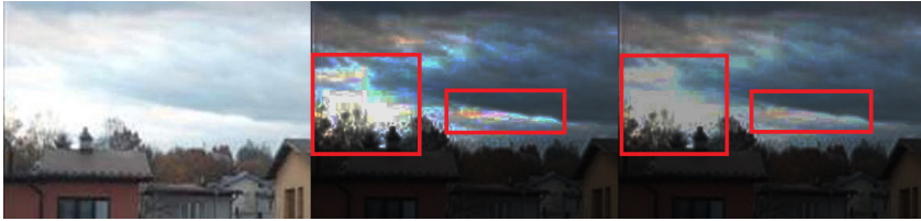
Figure 4.6: Illustration of the observed problem with increasing difference between color components. From the left to right: original image, under-exposed image with visible effect, and under-exposed image with compensated effect.
