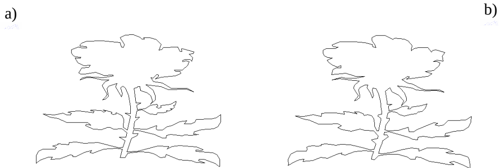
Fig. 3.25 Approximated Rose contour using a) Ramer method, and b) Analyzed method
