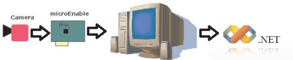
Fig. 6. General schema of the vision system connections
