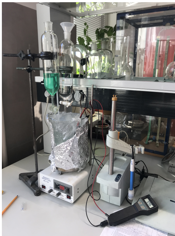
Figure 5.1. Co-precipitation setup for the synthesis of hydrotalcite-like catalysts with nickel. The solution is kept at a constant temperature of 50°C and stirred continuously with a magnetic stirrer. The precursor metals solution (green due to the nickel salt) and alkaline solution are poured dropwise and pH is monitored with a pH meter.
