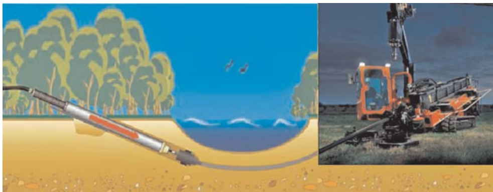
Rys. 1. Horizontal Directional Drilling
