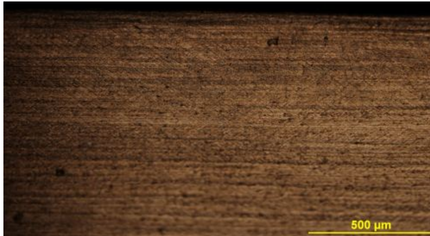
Figure 7.6. It is difficult micro shear bands aligned \pm 40^\circ to the rolling direction observed in parallel layers but aligned in an opposite manner.
