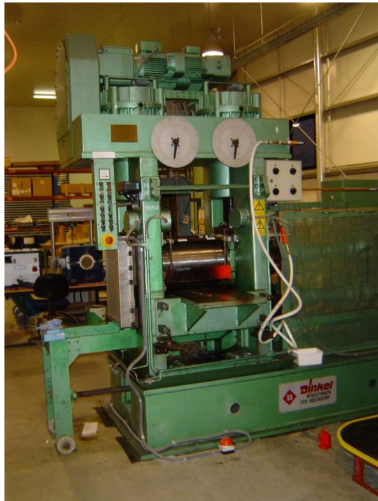
Figure 7.2. Two-high rolling mill used in the experiments.
