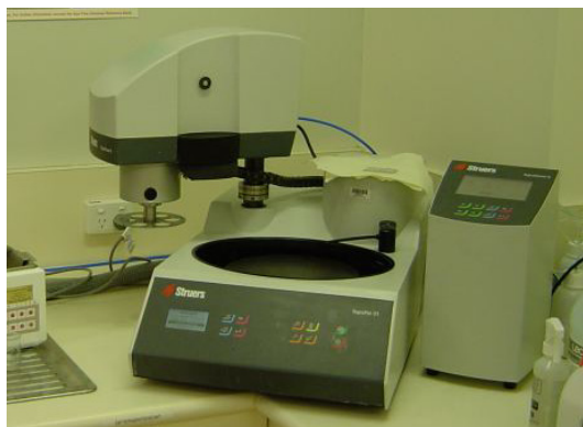
Figure 7.3. Manual and automatic polishing equipment available at the Center of Material and Fiber Innovation at Deakin University.
