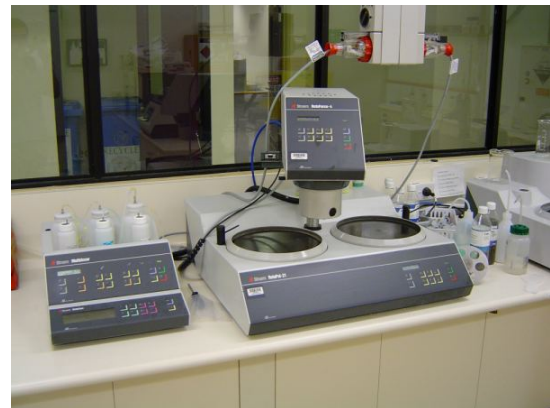
Figure 7.3. Manual and automatic polishing equipment available at the Center of Material and Fiber Innovation at Deakin University.
