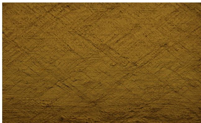
Figure 7.11. Highly visible crossing families of shear bands obtained for relatively low rolling reductions 50% + 5% additional rolling reduction.
