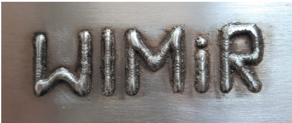
Fig. 7. A close-up image of the letters "WIMiR", hardfaced after establishing the right set of parameters
