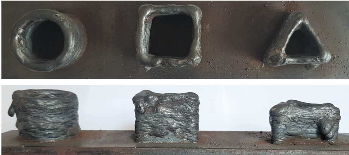
Fig. 8. The first trials of spatial hardfacing using the MIG/MAG method with the hardfacing machine
