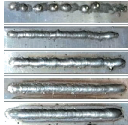
Fig. 5. Hardfacing trials at a current of 150 A
