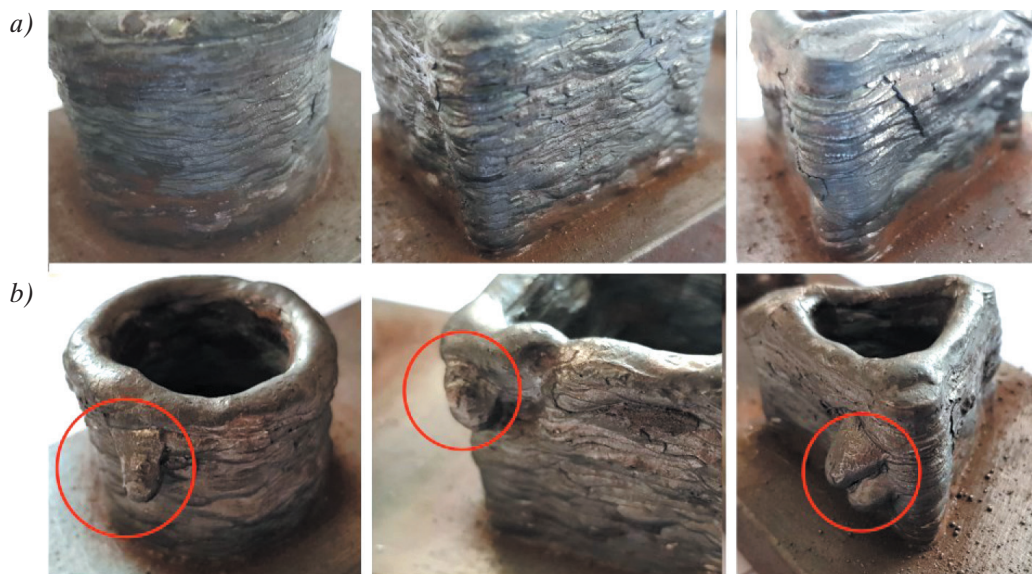
Fig. 9. Depicts correctly manufactured spatial hardfaced models (a); illustrates defects resulting from excessively high interlayer temperatures (b). The fragments with defects were not considered in the metrological verification
