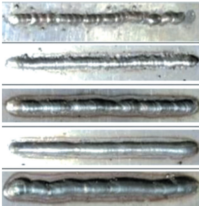
Fig. 4. Hardfacing trials at a current of 100 A. The best weld surface was achieved at a wire feed speed of 11.5 m/min
