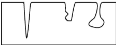
Figure 2.6. Morphology of pits
