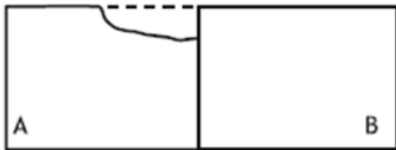
Figure 2.4. Galvanic corrosion on a seam of two metals.
