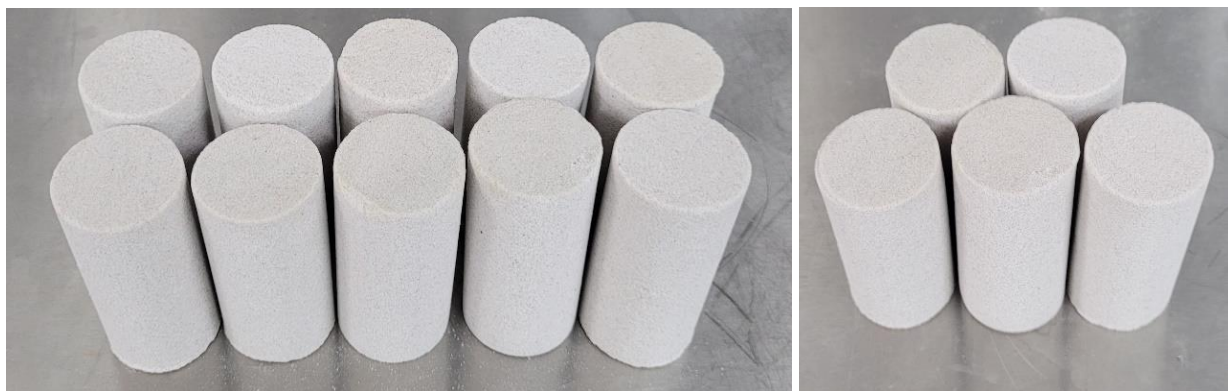
Figure 6.1: left) ten samples for measurement of rock's UCS; right) five samples for measurement of cohesion and internal friction angle of rock.
