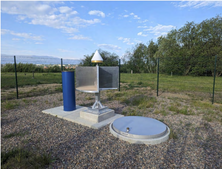
Fig. 1. Integrated ground monitoring station test setup at TU Bergakademie Freiberg (phot. J. Blachowski)
