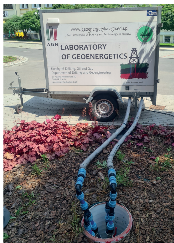
Fig. 1. TRT Equipment (photo Geoenergetics Lab team)
