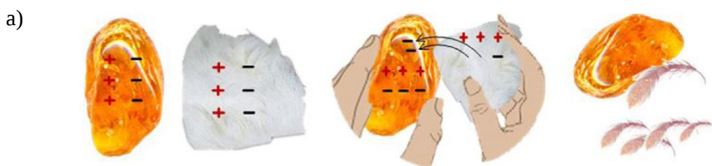
Fig. 2-2. Schematic diagram of electricity experiment with amber and cloth [32].
